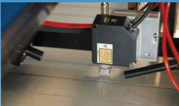
Ellipsometer & Eddy Current Head at the same point
